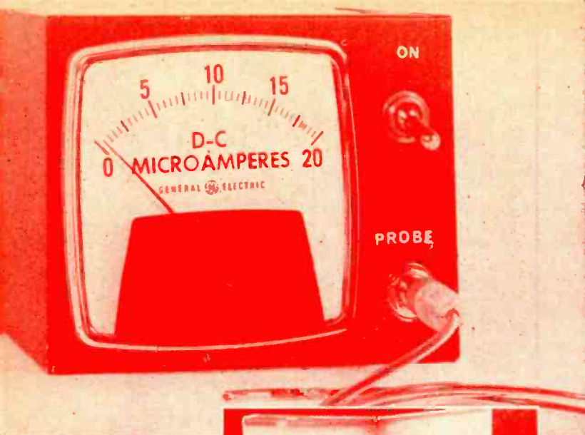
FRONT PANEL of the darkroom thermometer is plain and simple. Dial is calibrated in degrees for easy reading.
